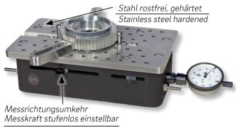
Reversible measuring direction Adjustable measuring force
